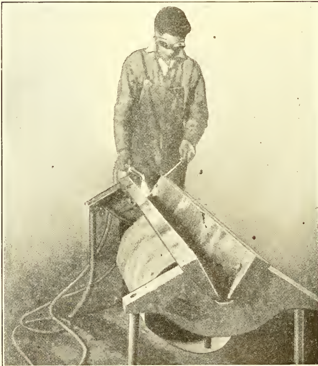
FIG. 186.—Large Sheet-Metal Cylinder Welding Jig.
